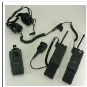
Figure 6: The two Motorola MX300 radio stations
