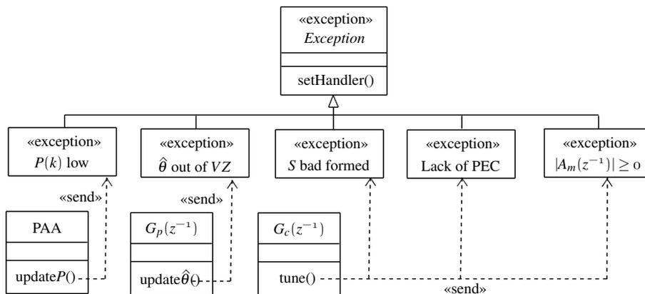
Figure 3: Modeling the exceptions of an adaptive control system
