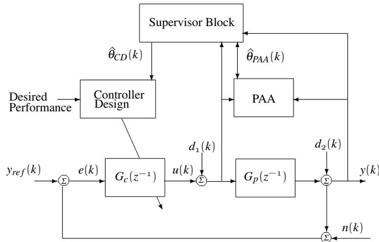
Figure 1: Indirect adaptive control system equipped with a supervisor block
