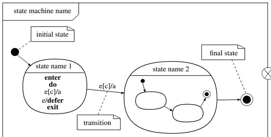
Figure 2: A state machine example
