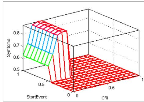
Figure 9: Three-dimensional trapezoidal membership function:  $Symptoms = f(CR_i, A_i)$
