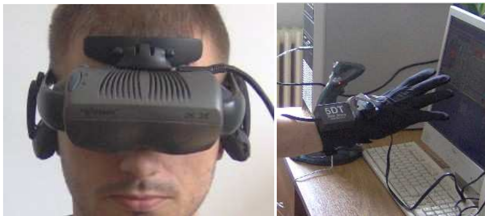
Figure 3: Using i-Glasses 3D and VR DataGlove to test the application at SSIB Suceava
