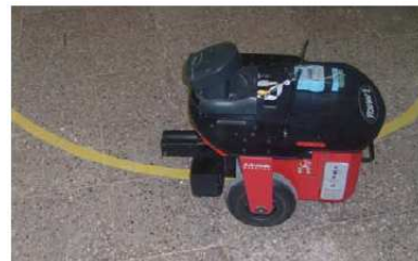
(b) Mobile robot Pioneer II DX used in our experiments.
