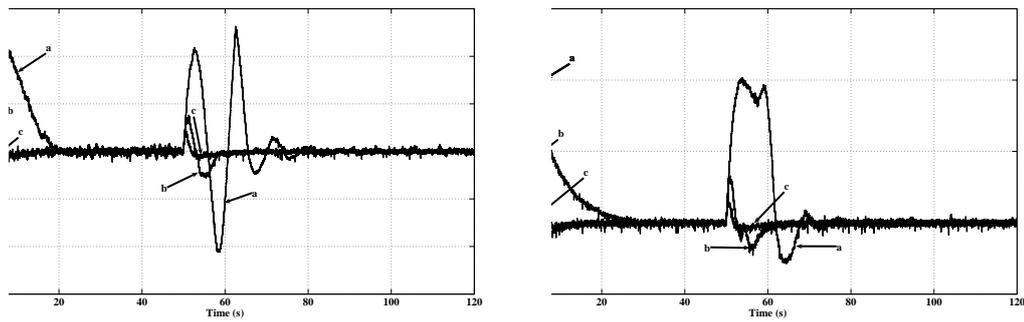
Figure 9: The errors  $e_1$  (left) and  $e_2$  (right) when using the gain scheduling controller (a), the linear parameter varying controller (b) and the input-output feedback linearization controller (c)
