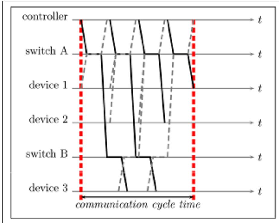
Figure 11: EtherNet/IP space-time diagram for 4-ports switches
