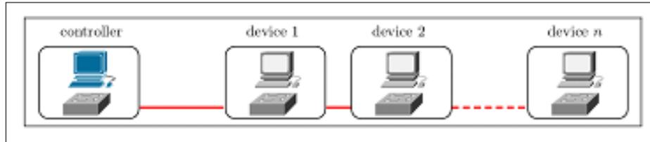
Figure 5: Profinet line topology
