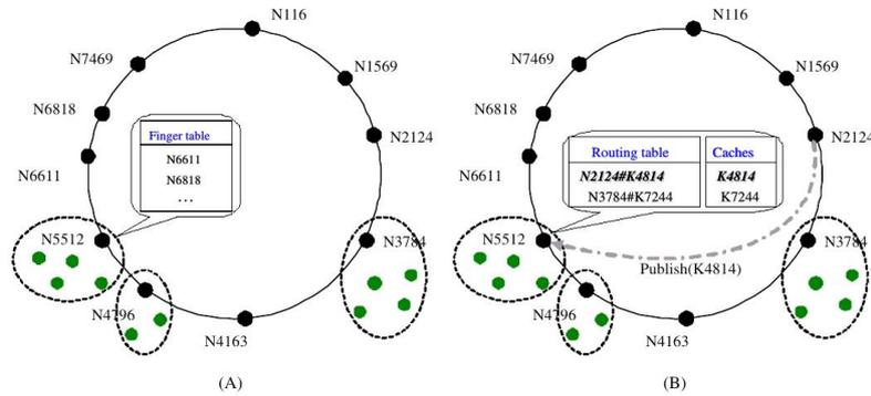
Figure 3: (A) Finger Table of  $N5512$ ; (B) Routing Table and Cache Table of  $N5512$
