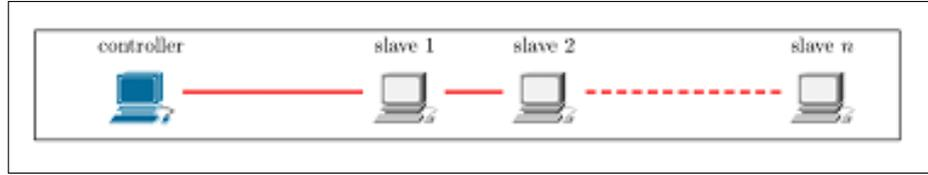
Figure 3: EtherCAT line topology
