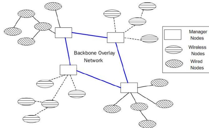
Figure 1: The Topology of Wireless/Wired Mixed Network via MBRP
