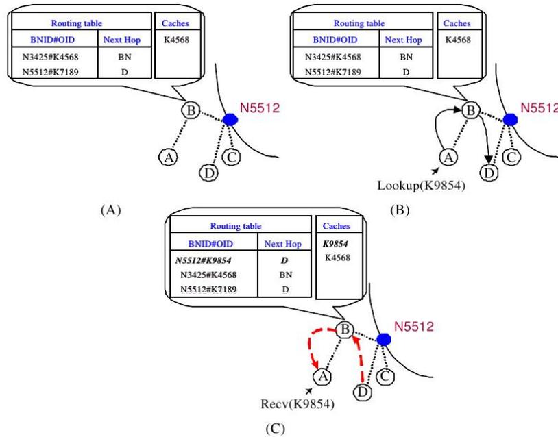
Figure 4: (A) Routing Table of Internal Node B; (B) Lookup Originated from Internal Node A to B and D; (C) Lookup Succeed Message Passed Back From D to B and A
