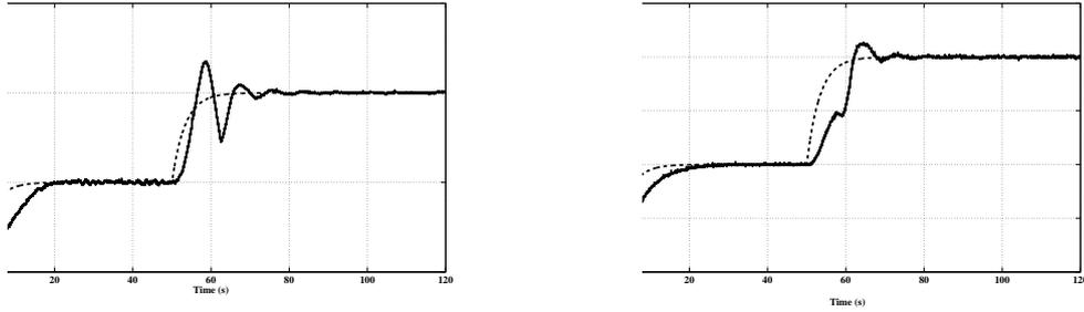
Figure 3: The water levels of tank 1 (solid: left) and tank 2 (solid: right) when using the gain scheduling controller. The references  $r_1$  and  $r_2$  are depicted using the dashed lines
