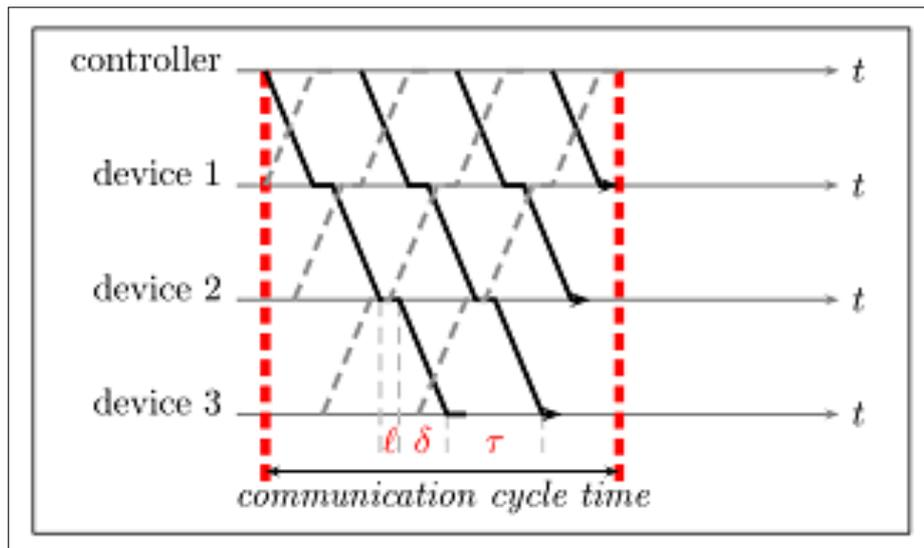
Figure 6: Profinet IRT space-time diagram with *slipstreaming effect*
