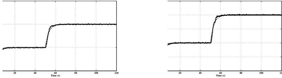
Figure 5: The water levels of tank 1 (solid: left) and tank 2 (solid: right) when using the linear parameter varying controller. The references  $r_1$  and  $r_2$  are depicted using the dashed lines
