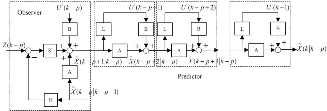
Figure 1: Block diagram of the delay compensation algorithm.
