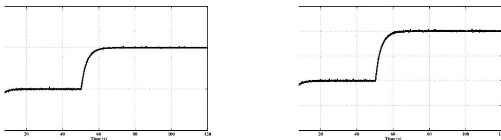
Figure 7: The water levels of tank 1 (solid: left) and tank 2 (solid: right) when using the input-output feedback linearization controller. The references  $r_1$  and  $r_2$  are depicted using the dashed lines
