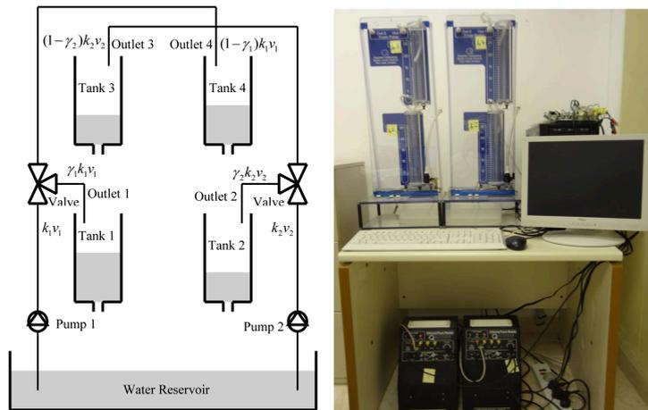
Figure 1: A schematic diagram (left) and a picture (right) of the quadruple tank process
