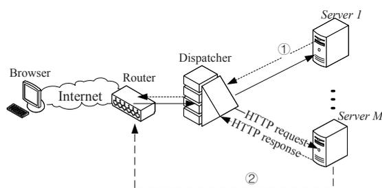
Figure 1: The Processing of HTTP Request in Web Cluster
