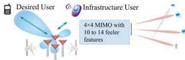
Figure 2: Beamforming for Long-Term Evolution and IEEE 802.16 standard devices
