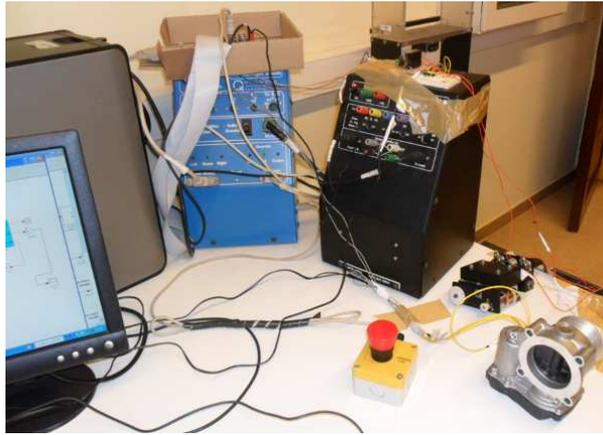
Figure 3: Laboratory testbed. Experimental setup for controlling the electronic throttle: Quanser power amplifier, Quanser real-time control board, and ETB.
