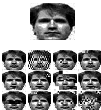
Figure 2: Effect of soft-errors for the decoding of JPEG files. (a) Decoded image without soft-errors (b) Examples of decoded images with bit-errors
