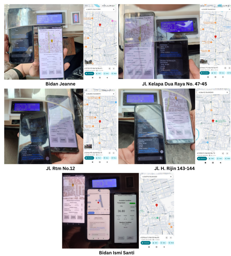
Figure 11: Received SMS from the portable neonatal incubator alert system with Google Maps web page from accessing the URL stated on the SMS
