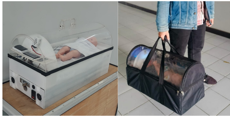
Figure 8: The prototype of portable neonatal incubator with the carrying bag
