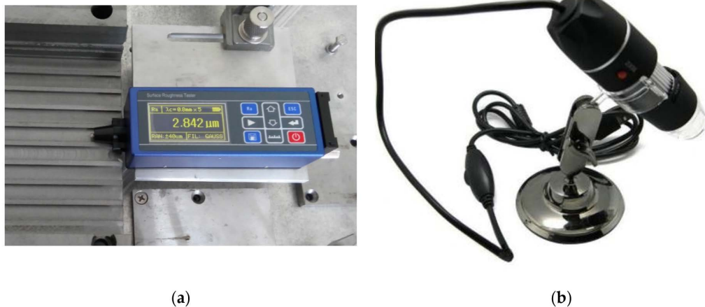
Figure 3: Pictures of equipment used: (a) Surface Roughness Tester; (b) Digital Microscope 50x.
