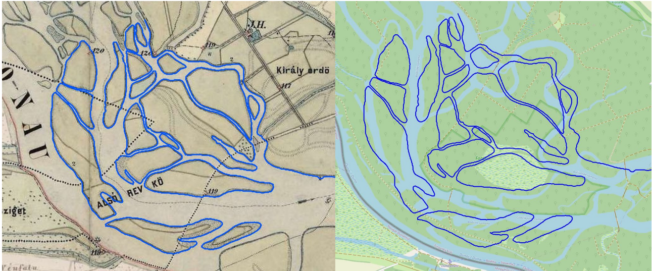
Figure 7: The segmentation of a part of the Danube branch system around the Bodické Rameno performed on historical maps from the Third Military Survey (left), transformed to OpenStreetMap using the LAGL algorithm [19] (right). Data source: Historical map of the Third Military Survey in raster form (GKÚ Bratislava, NLC) and OpenStreetMap.
