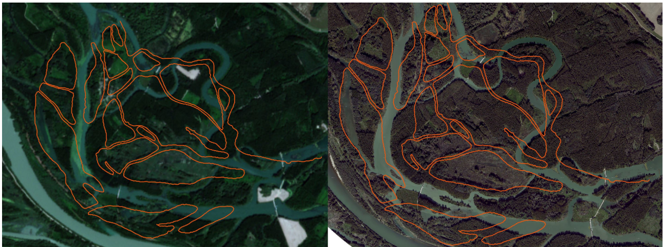
Figure 8: The transformed segmentation of a part of the Danube branch system around the Bodické Rameno is positioned over Sentinel-2 data (left) and an orthophotomosaic image (right). Data source: Sentinel-2 L2A product acquired on 30 July 2024 (Copernicus Data Space Ecosystem, ESA) and Orthophotomosaic of Slovakia from 2020 (GKÚ Bratislava, NLC).
