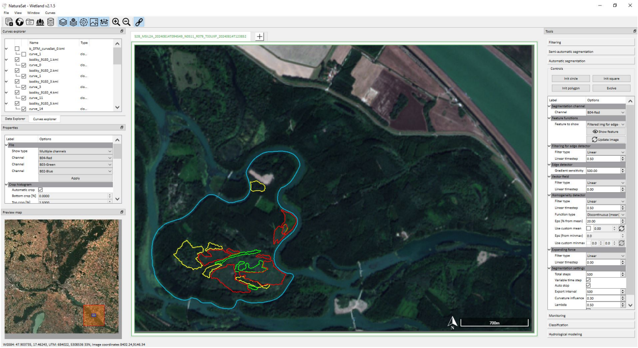
Figure 2: The user interface of the NaturaSat software with loaded Sentinel-2 data and highlighted segmentation polygons. Data source: Sentinel-2 L2A product acquired on 14 August 2024 (Copernicus Data Space Ecosystem, ESA)
