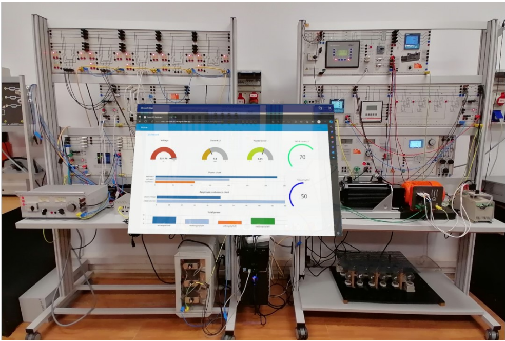
Figure 6: Augmented XR HMI seen from Hololens Industrial headset.
