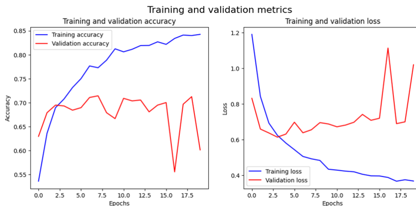
Figure 4: Accuracy and loss of training and validation metrics for ResNet152V2
