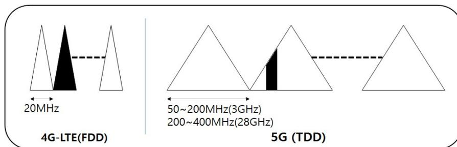
Figure 4: Comparison between FDD and TDD [8]
