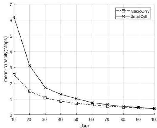
Figure 10: Capacity comparison when 5G macro communication and small cell are applied
