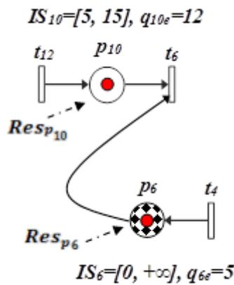
Figure 4: Study of constraints violation at the synchronization transition  $t_6$
