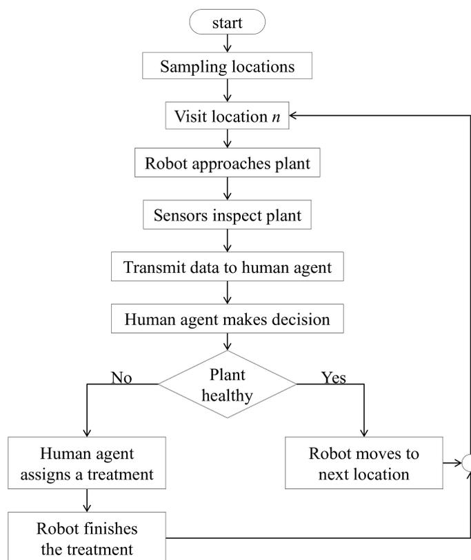
Figure 2: Agricultural Robotic System (ARS) work operations
