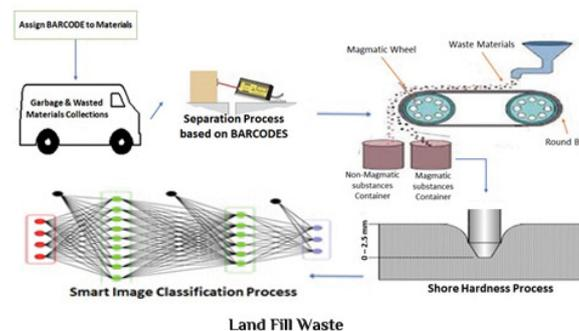
Figure 5: Semi Smart Trash Separator proposed approach
