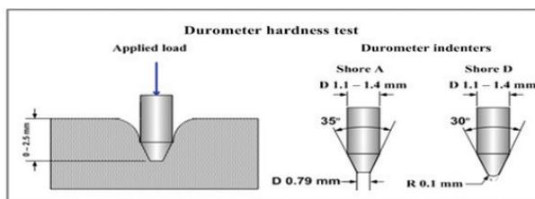
Figure 7: Soft material durometer hardness test
