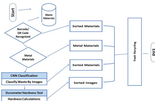
Figure 6: Semi smart trash separator stages
