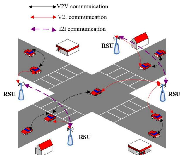
Figure 1: Schematic diagram of VANET road communication
