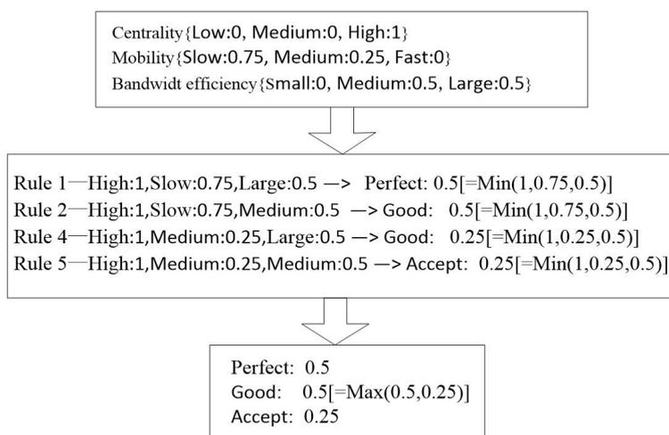
Figure 7: Example of Fuzzy Logic rule mapping
