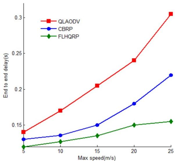
Figure 15: Comparison of average end to end delay
