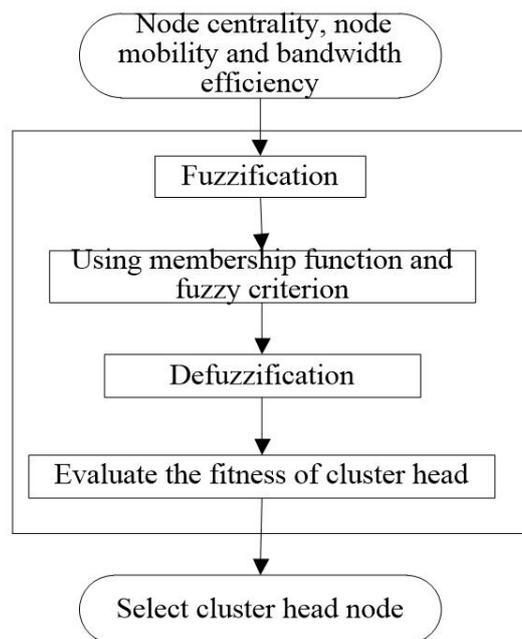
Figure 3: Steps of selecting a CH based on Fuzzy Logic
