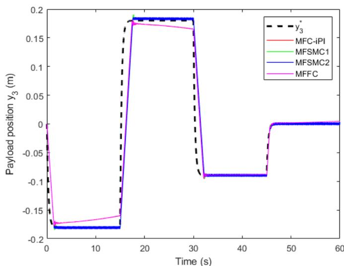
Figure 6: The experimental results of the CS with MFC-iPI, MFSCM1, MFSCM2 and MFFC controllers expressed as reference trajectory and controlled outputs (payload position) versus time
