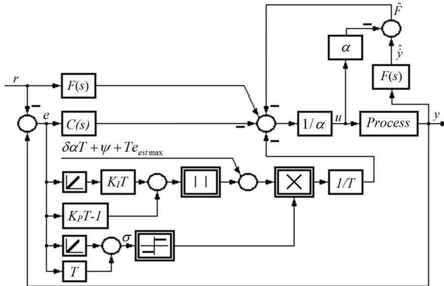
Figure 3: Control system structure with second data-driven model-free sliding mode controller [57]
