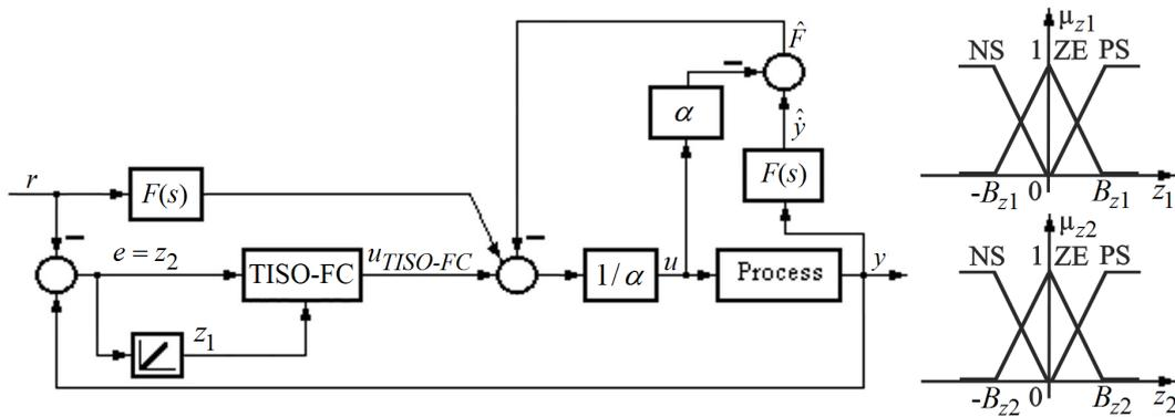
Figure 4: Control system structure with data-driven model-free fuzzy controller and input (scheduling) membership functions
