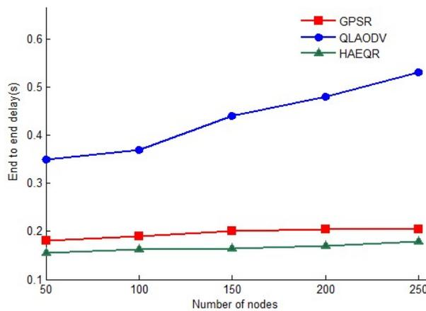
Figure 8: Comparison of end-to-end delay of different vehicle nodes.
