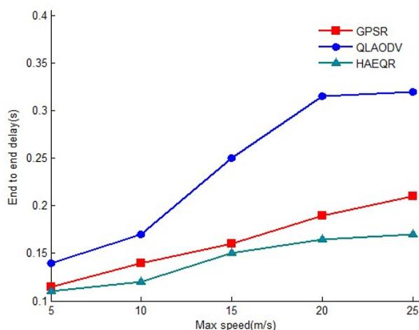
Figure 11: Comparison of end-to-end delay at different moving speeds.
