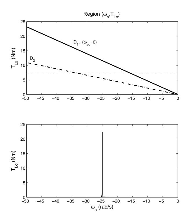
Figure 6: A proposed observer design was used. First subplot shows region  $(\omega_o, T_{Lo})$  with the line  $D_1 = D_3$ . Second subplot shows the actual angular speed.
