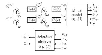
Figure 4: Block diagram of sensorless RFOC induction motor simulator.
