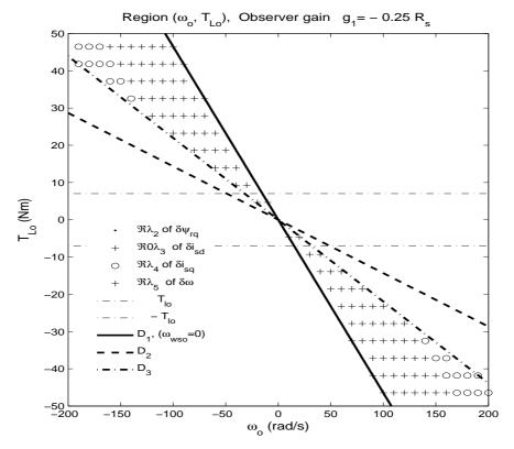
Figure 3: Torque/speed plane,  $g_1 = -0.25R_s$ ,  $\Re(\lambda_i) > 0, i = 1...5$
