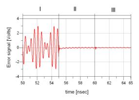
Figure 4: The error between both signals provided by the oscillators
