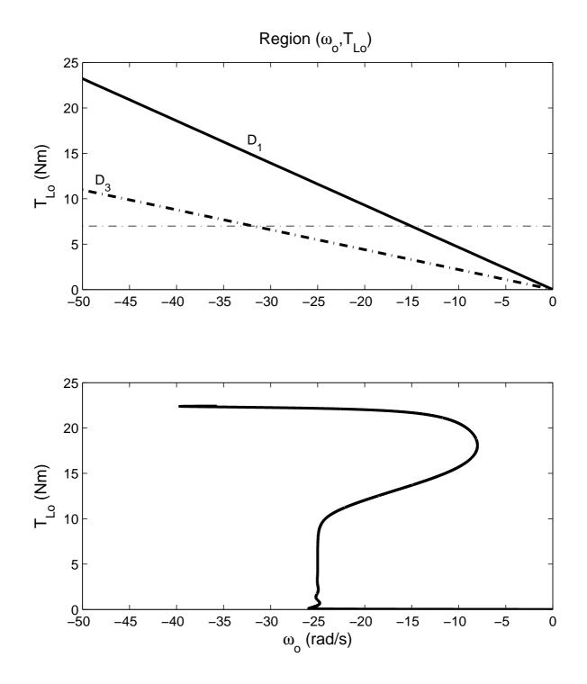
Figure 5: A rated-load torque ramp is applied with the observer gain  $g_1 = -0.25R_s$ . First subplot shows region ( $\omega_o, T_{Lo}$ ) with the two lines  $D_1$  and  $D_3$ . Second subplot shows the actual angular speed.
