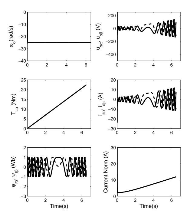
Figure 8: The instability was removed by the proposed observer design  $g_1 = -L_r R_s / L_m$ .
