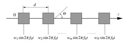
Figure 1: An uniform antenna array
