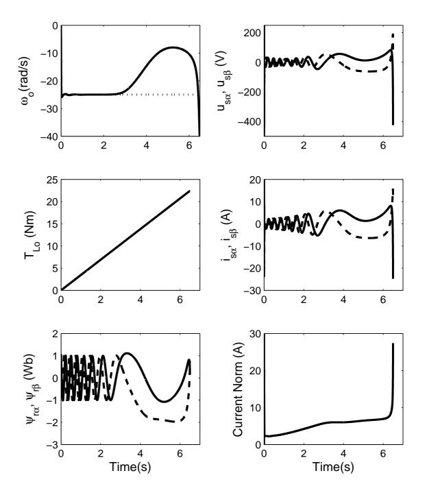
Figure 7: Instability phenomenon with observer gain  $g_1 = -0.25R_s$ .
