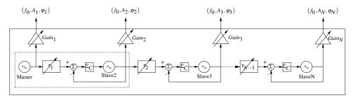
Figure 2: Unidirectional coupling of a chain of oscillators
