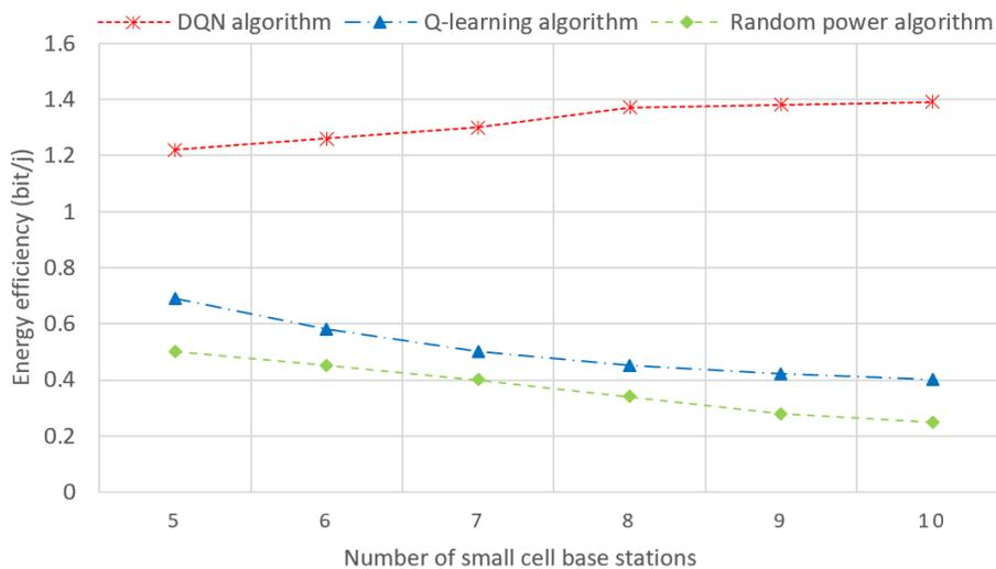
Figure 3: Energy efficiency at different numbers of base stations
