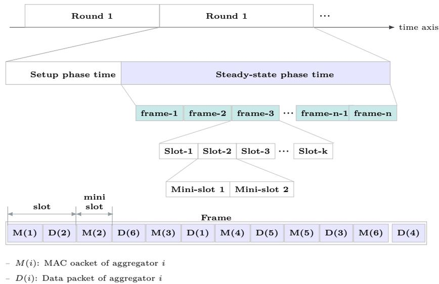
Figure 5: The proposed TDMA for the aggregators transmission
