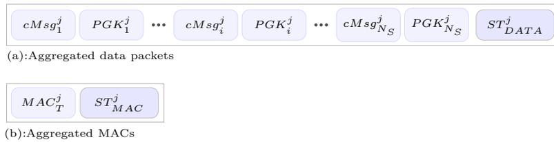
Figure 4: Aggregated packets for CA of cluster  $j$
